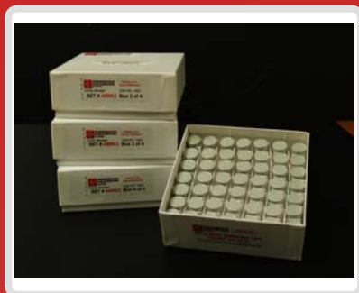
Referee Level Particle Standards (RLPS™) with NIST Traceable Single Seed Particle per Container
